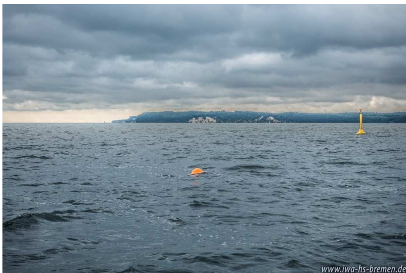
Fig. 12. Wave measurements with miniature wave buoy in the Prorer Wick, Island of Rügen, Germany.
